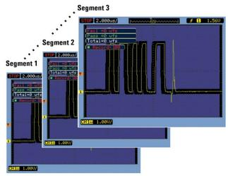
Figure 6 — Using Sequence mode in combination with mask testing on the Agilent 1000 Series oscilloscope to record and capture 1000 trigger occurrences.
