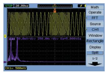
Figure 3 — Input sine wave shown on top half of the screen and the FFT analysis shown in the lower half of the screen on an Agilent 1000 Series oscilloscope.
