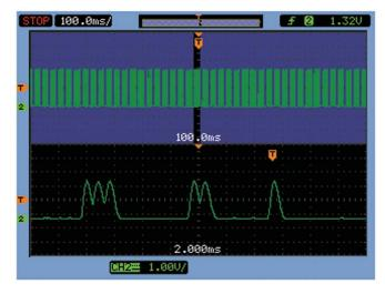
Figure 1. An example of a long acquisition utilizing the 20 kpts of memory on the Agilent 1000 Series oscilloscope.
