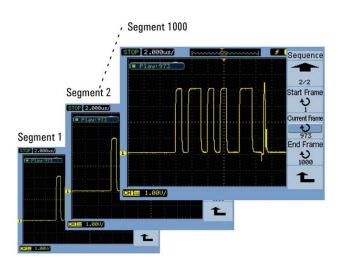
Figure 4. Use sequence mode to record up to 1000 triggers and review in playback mode for anomalies.
